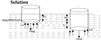
At equilibrium, upthrust of the liquid on the rod is equal to the weight of the displaced fluid
