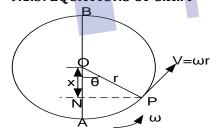
Consider a particle, p of mass, m, moving round a circle of radius, r, with uniform angular velocity,  $\omega$ , . Let the particle be at point p, t seconds after starting motion from A such that the angle subtended at the centre is  $\theta$
