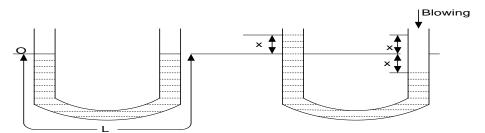
When the meniscus is at a distance, x, from equilibrium position, a differential height of liquid of, 2x, is produced
