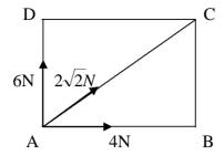
Three forces act along AD, AB and AC as shown above. ABCD is square. Determine the resultant of the three forces and the angle which it makes with AB.
